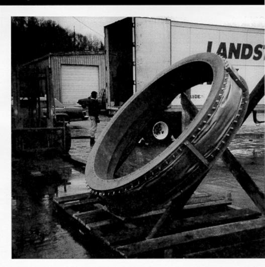
Pair of angle frame round expansion joints with one liner.
